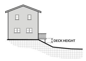
FIGURE 18.02.030.C.2: MEASURING HEIGHT OF DECKS
