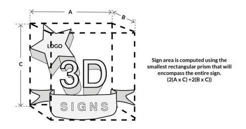
FIGURE 18.18.050.A.4: MEASURING SIGN AREA, 3D SIGNS
