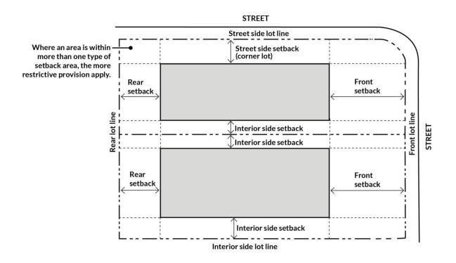
FIGURE 18.02.030.I: DETERMINING SETBACKS
